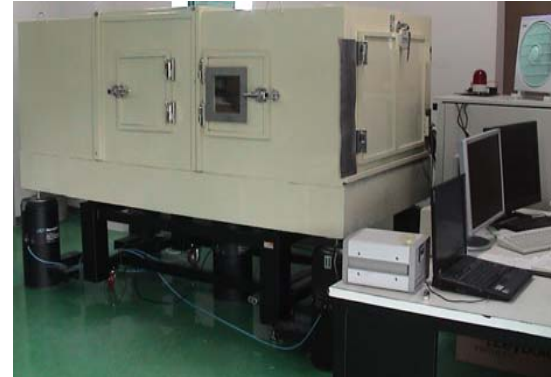
Phase Contrast X-ray Radiography - Non destructive test
